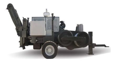
The machine allows for the tension stringing of 4-bundle conductor of 630mm² and below in mountainous and hilly areas, and of 4-bundle conductor of 720mm² and below in flat lands; besides, it can be used for traction stringing of OPGW or ADSS optical cable and 500kV traction stringing in various terrains.
