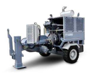
This machine allows for the tension stringing of twin-bundle conductor of 500mm² and below in mountainous and hilly areas, of twin-bundle conductor of 630mm² and below in flat lands, and of single conductor 720mm² in various terrains; besides, it can be used for traction stringing of OPGW or ADSS optical cable and 220kV haulage rope in various terrains.
