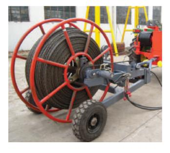
The reel winders are suitable to work with any hydraulic power unit, in particular with pullers and puller-tensioners, and operate as separated winding systems. They are equipped with automatic level wind and negative self-acting hydraulic brake. The frame is made of welded steel with protective coating. The reel winders can lift the reel by hydraulic jacks powered by the same hydraulic source.
