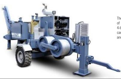
The machine allows for the tension stringing of 4-bundle conductor of 630mm<sup>2</sup> and below in mountainous and hilly areas, and of 4-bundle conductor of 720mm<sup>2</sup> and below in flat lands; besides, it can be used for traction stringing of OPGW or ADSS optical cable and 500kV traction stringing in various terrains.
