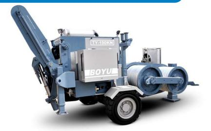
The machine allows for the tension stringing of 4-bundle conductor of 630mm<sup>2</sup> and below in mountainous and hilly areas, and of 4-bundle conductor of 720mm<sup>2</sup> and below in flat lands; besides, it can be used for traction stringing of OPGW or ADSS optical cable and 500kV traction stringing in various terrains.
