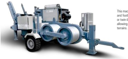
This machine is mainly applied in long-span and mountainous areas and foothills for tension stringing of 4-bundle conductor of 500kV or twin-bundle conductor of 220kV and conductor 800mm<sup>2</sup> below, allowing for the tension stringing of 500kV haulage rope in various
