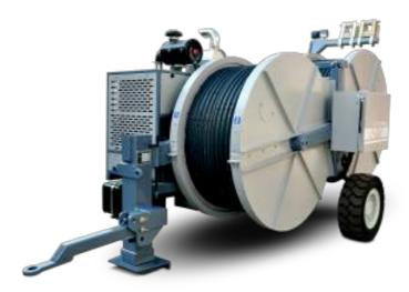
The machine allows for the tension stringing of twin-bundle conductor of 630mm² and below in mountainous and hilly areas, of twin-bundle conductor of 720mm² and below in flat lands, and of conductor 720mm² in various terrains; besides, it can be used for tension stringing of OPGW or ADSS optical cable and 500kV haulage rope in various terrains
