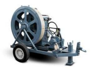
Applied for tension stringing of the transmission line conductors and ground cables, and ADSS, OPGW optical cables.
