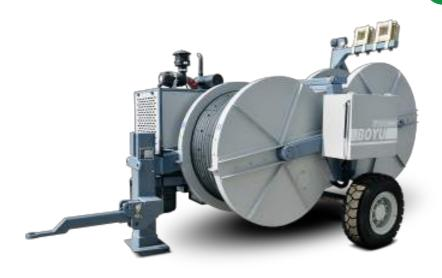
The machine allows for the tension stringing of twin-bundle conductor of 630mm<sup>2</sup> and below in mountainous and hilly areas, of twin-bundle conductor of 720mm<sup>2</sup> and below in flat lands, and of conductor 720mm<sup>2</sup> in various terrains; besides, it can be used for tension stringing of OPGW or ADSS optical cable and 500kV haulage rope in various terrains
