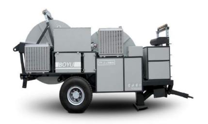
The machine allows for the tension stringing of twin-bundle conductor of 630mm<sup>2</sup> and below in mountainous and hilly areas, of twin-bundle conductor of 720mm<sup>2</sup> and below in flat lands, and of 1 conductor 720mm<sup>2</sup> in various terrains; besides, it can be used for tension stringing of OPGW or ADSS optical cable and 500kV haulage rope in various terrains
