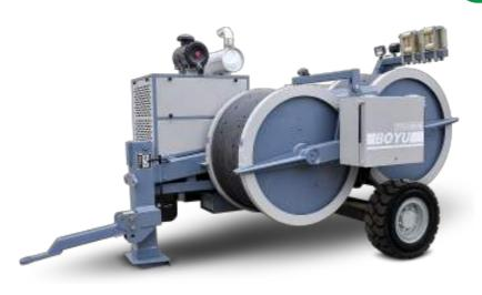
The machine allows for the tension stringing of twin-bundle conductor of 630mm<sup>2</sup> and below in mountainous and hilly areas, of twin-bundle conductor of 720mm<sup>2</sup> and below in flat lands, and of conductor 720mm<sup>2</sup> in various terrains; besides, it can be used for tension stringing of OPGW or ADSS optical cable and 500kV haulage rope in various terrains
