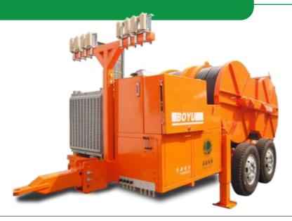
The machine allows for the tension stringing of max 4-bundle conductor of 630mm² and below in mountainous and hilly areas, of max 4-bundle conductor of 720mm² and below in flat lands, and of 2 conductor 720mm² in various terrains; besides, it can be used for tension stringing of OPGW or ADSS optical cable and 500kV haulage rope in various terrains
