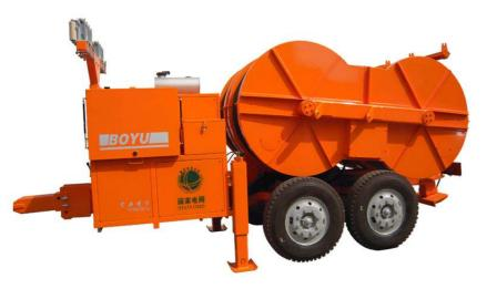
The machine allows for the tension stringing of one, two, three or four-bundle conductor of 630mm2; besides, it can be used for tension stringing of OPGW or ADSS optical cable and 500kV haulage rope in various terrains, suitable for use at altitudes up to 1500 meters above sea level.
