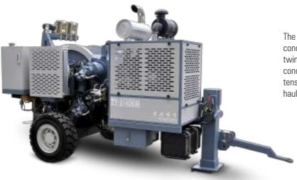
The machine allows for the tension stringing of twin-bundle conductor of 630mm² and below in mountainous and hilly areas, of twin-bundle conductor of 720mm² and below in flat lands, and of conductor 720mm² in various terrains; besides, it can be used for tension stringing of OPGW or ADSS optical cable and 500kV haulage rope in various terrains
